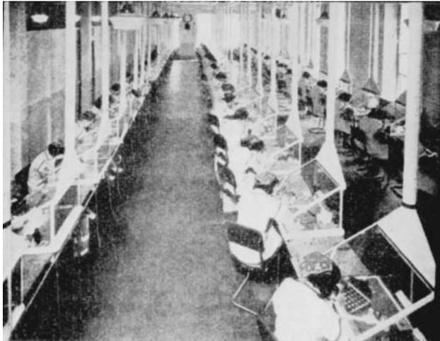
**Figure 3** Radium dial painting operation after implementation of industrial hygiene measures including banning of oral “tipping” of brushes and construction of ventilated work enclosures (Hunter 1969)
